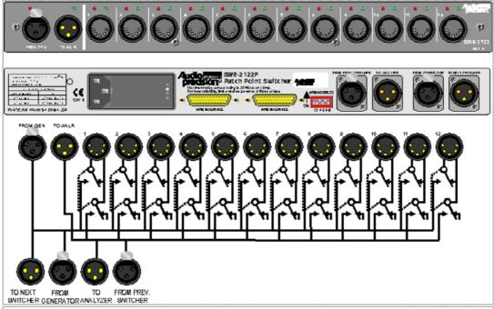
SWR-2122P Patch-Point Switcher. 12 point configuration allows a signal path to be interrupted and a test generator inserted while a measuring analyzer can access the output of a previous device. In the default (non-accessed) mode, the path continuity is maintained. Each of the 12 insertion points is provided with a 5-pin XLR connector to allow balanced interface to previous and next device.
